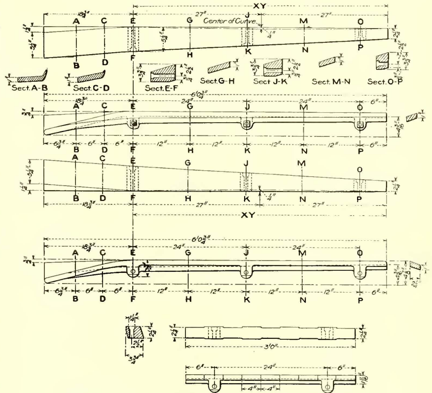
Brooklyn Line Department—Third-Rail Switch Wings, Right and Left
