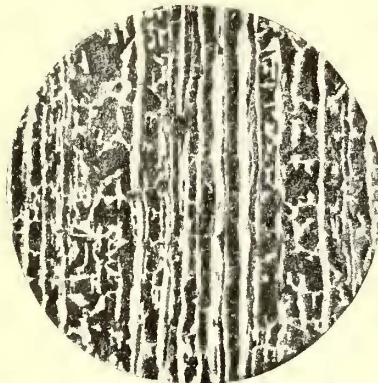
Fig. 2—Structure of Old Corrugated Rail
