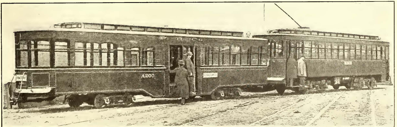
Pittsburg Trailer Operation—View of Motor and Trail Car Illustrating the Respective Places for Boarding and Alighting, Except That the Front Exit of the Motor Car Is Not Shown in Use
