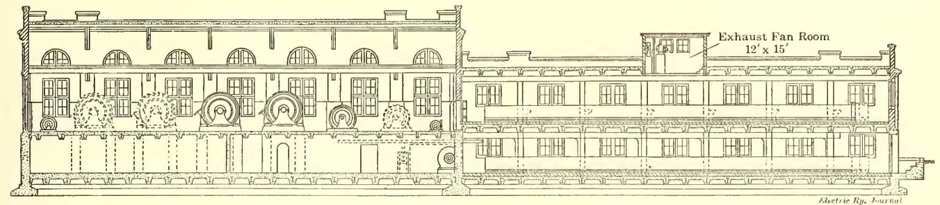
Fig. 9—Detroit Tunnel—Longitudinal Section Along the Line H-H on the Plan of Substation
