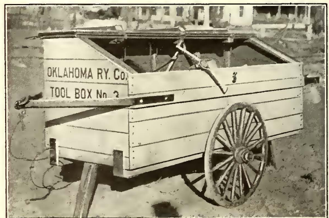
Fig. 14—Oklahoma Track—Portable Tool Box Used by Small Construction Gangs
