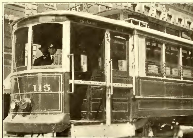
Platform Bar in Service Position
