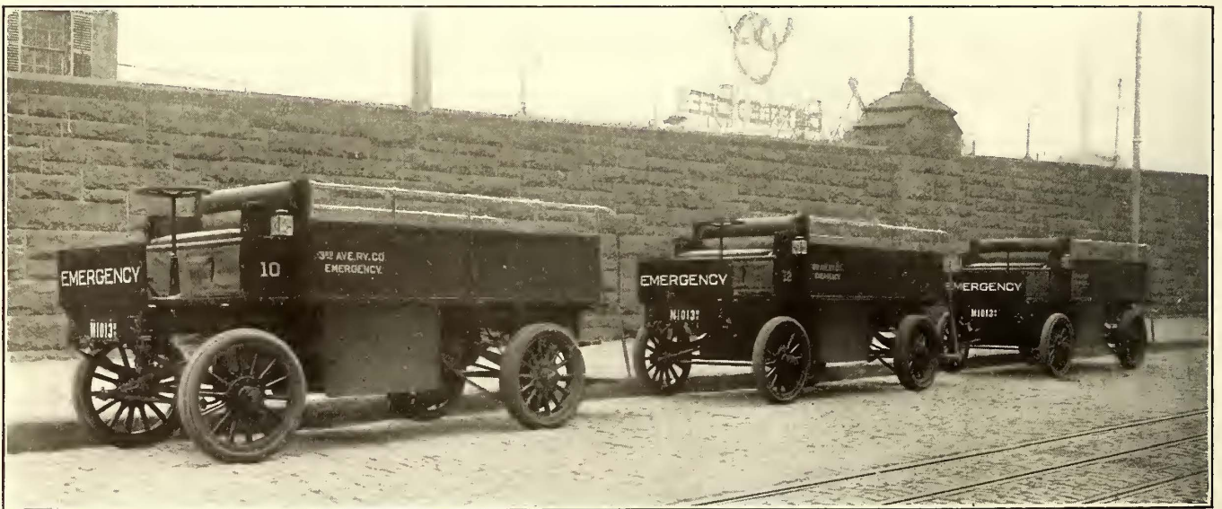
Three Electric Emergency Wagons for Third Avenue Railroad, New York
