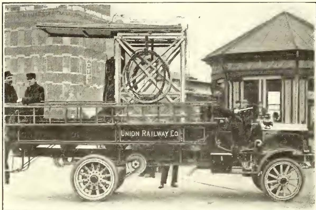
One of Four Gasoline Tower Auto-Trucks for the Union Railway, New York
