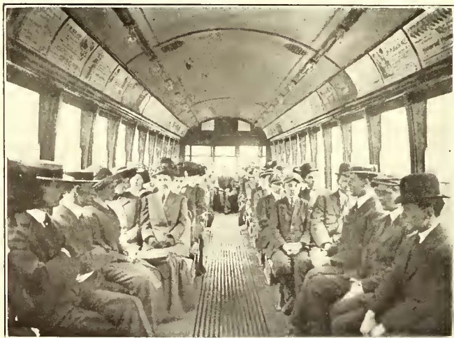
Near-Side Car—Interior View Showing Longitudinal Seats in Front, Circular Seating at Rear and Cross Seats
