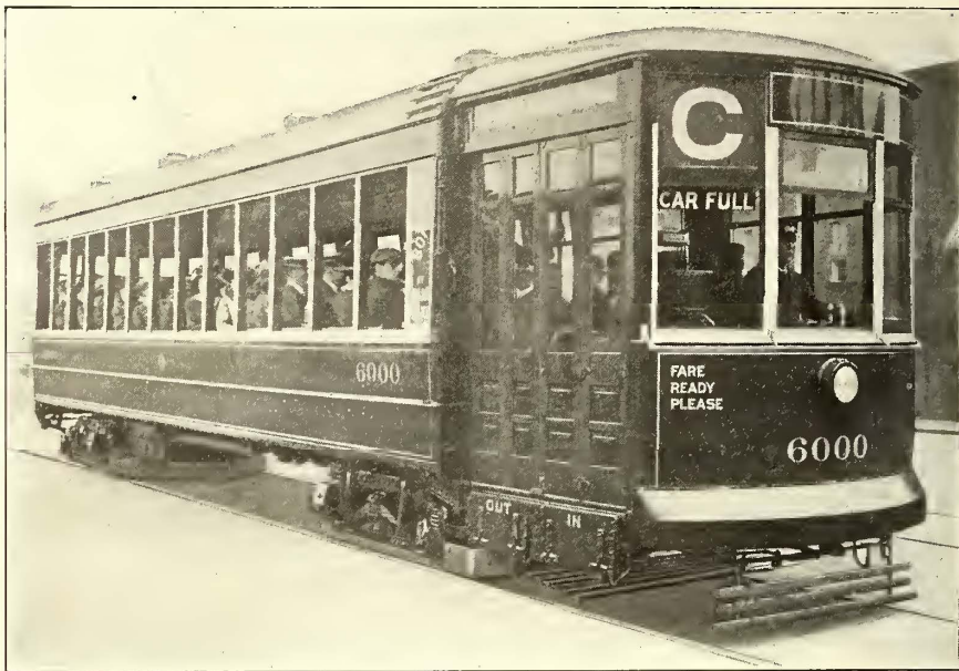
Near-Side Car—View Showing Closed Doors and Folded Steps on Front Platform, Front and Side Destination Signs, "Car Full" Sign, Etc.
