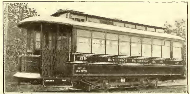
Cab-on-Platform Car for Hutchinson, Kan.
