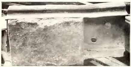
Side View and Sectional View of Old Cast-Welded Rail Joints
