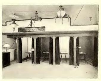
Compartments in the Basement for Testing the Absorption of Light by Wall Papers of Different Colors
