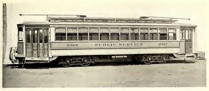
Exterior View of 2300 Class Double-End Closed Car
