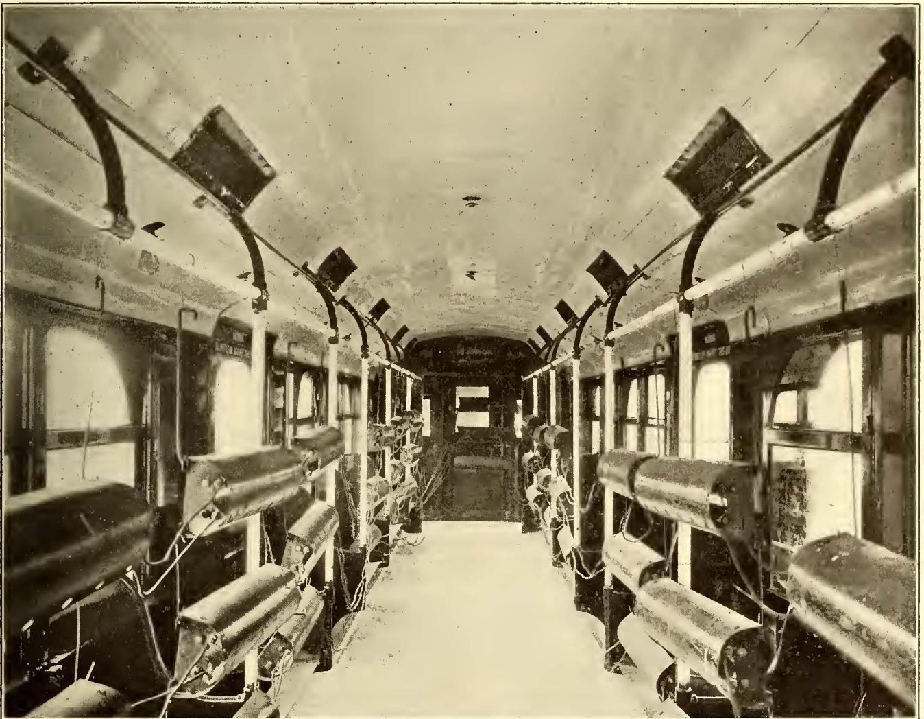
Hudson & Manhattan Painting—View of Interior of Car After Completion of Baking Process, Showing Electric Heaters Hung from the Hand Rods
