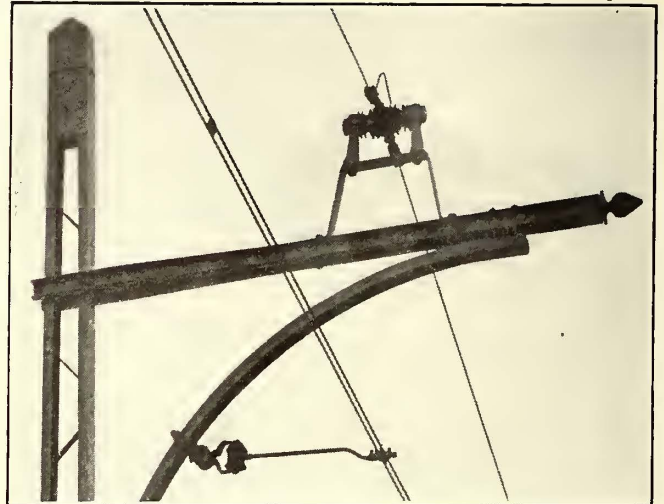
Leyden-Katwyk-Noordwyk Railway—Loop in Copper Catenary, and Idle Trolley Wire Clipped to Active One
