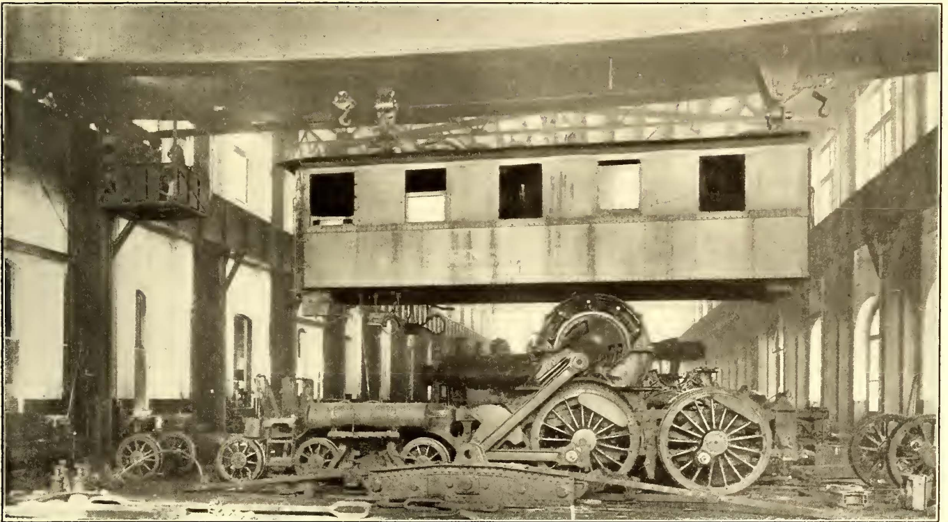
Pennsylvania Locomotives—View of Crane in Meadows Shop Lifting Cab from a Unit.
