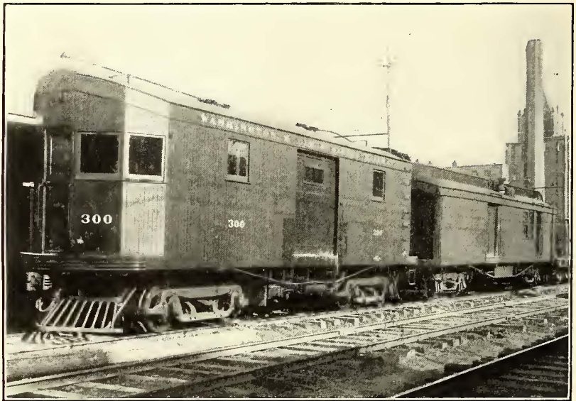
Washington & Old Dominion Railway—Overhead Construction and Freight Motor Car with Standard Railroad Baggage and Mail Car
