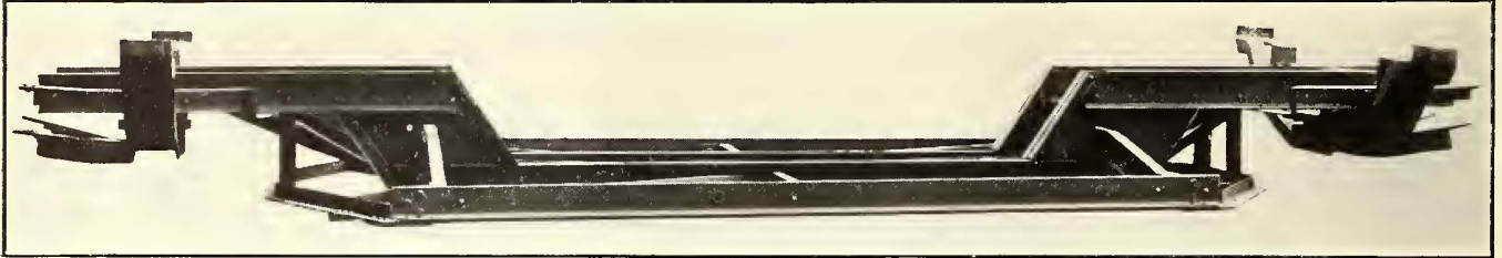
Improved Articulated Car—View of Framing for Central Section Showing Offset in Center Sills and Method of Supporting Side Sills
