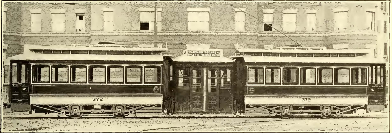
Improved Articulated Car—General View Showing New Arrangement of Central Section with Stepless Feature
