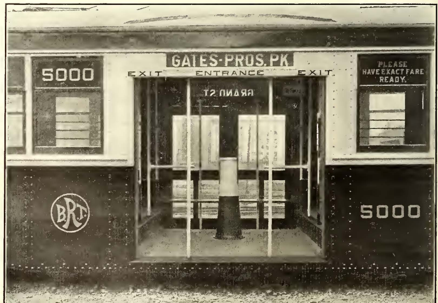
Brooklyn Center-Entrance Car—Detail at Center Entrance, Showing Dividing Rails and Stanchions, Conductor's Pedestal, Downwardly Swiveled Seats Alongside Closed Doors, Signs, etc.
