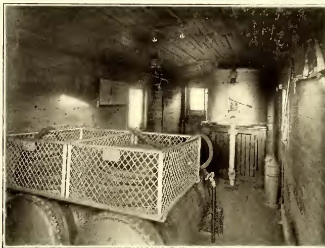
Fire Engine Car—Interior View, Showing Hose Racks and Tanks
