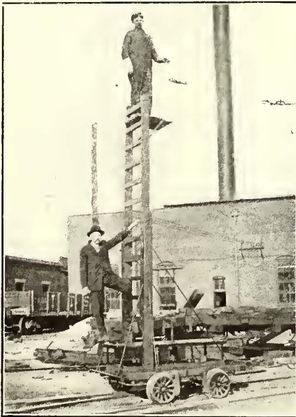
Illinois Traction System—Extension Ladder on Gasoline Line Car
