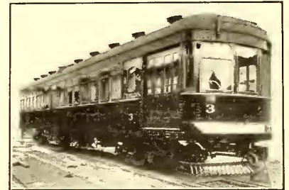
Pacific Coast Car—Side and End Views Showing Drop Siding and End Doors for Baggage
