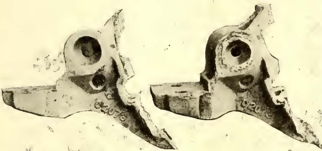
San Francisco Shops—Brakehead with Worn Socket Before and After Repair
