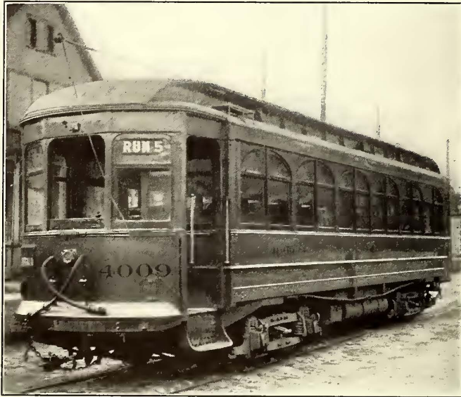
Buffalo Car Maintenance—City Car as Rebuilt for Interurban Service on Lockport Line
