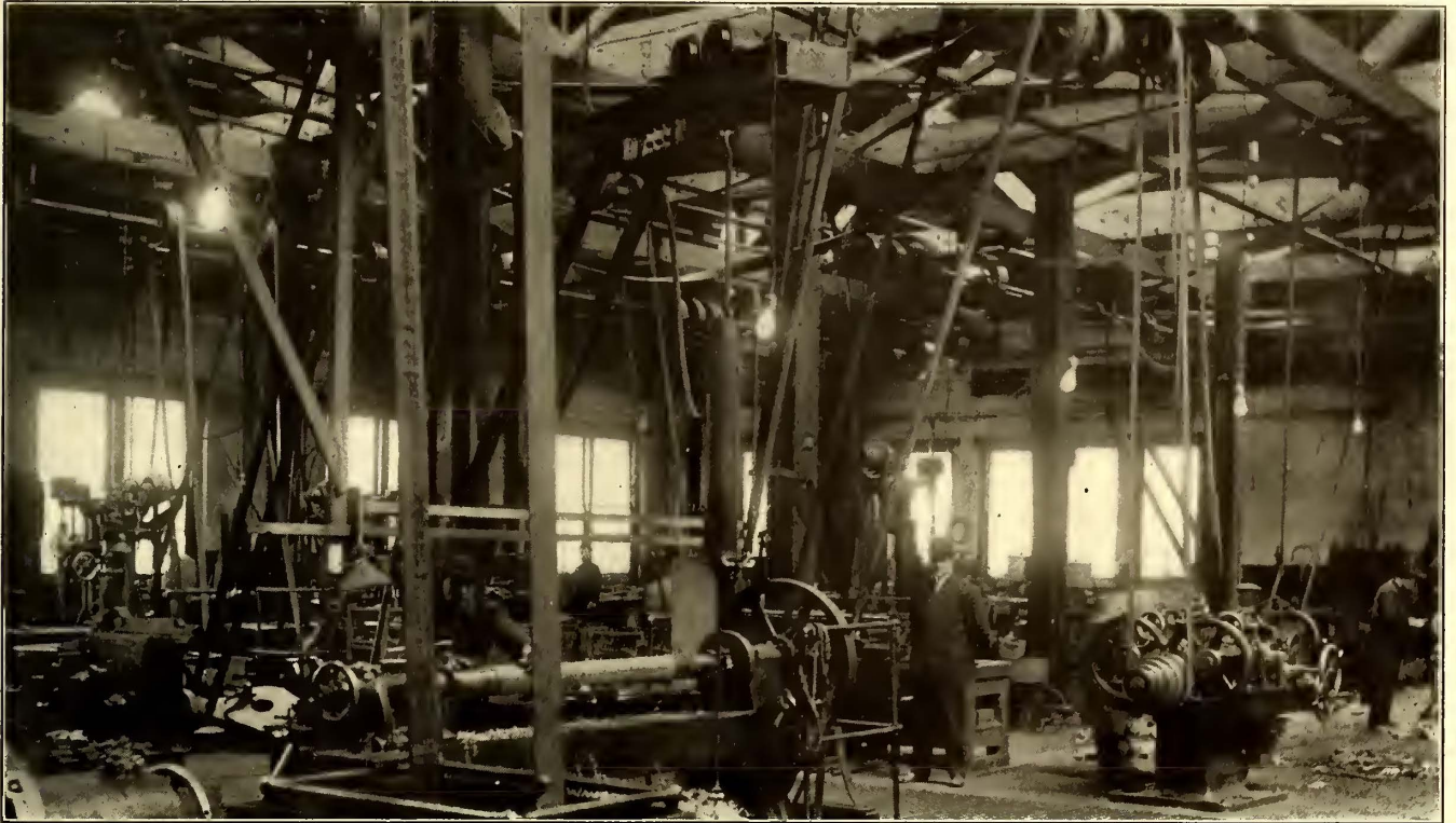
Buffalo Car Maintenance—View of Corner of Cold Spring Machine Shop, Showing Air Lift and Jib Crane Used for Handling Axles
