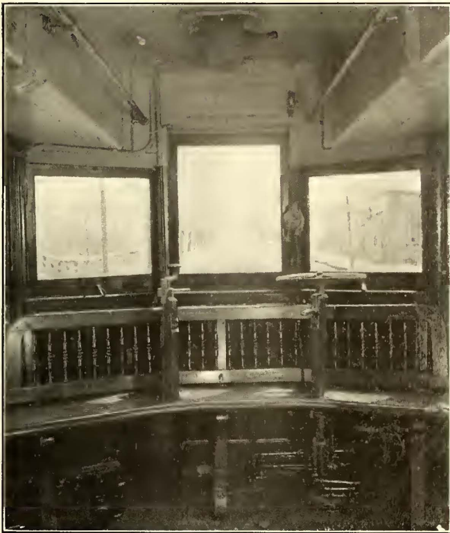
Pittsburgh Double-Deck Cars—View Showing Controller Under Stationary End-Seat with Extended Shaft for Operating Handle
