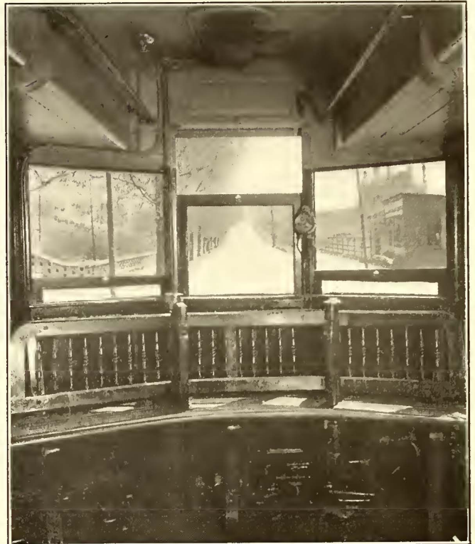
Pittsburgh Double-Deck Cars—View at Rear End Showing Controller and Brake Handles Removed to Provide Room for Seated Passengers
