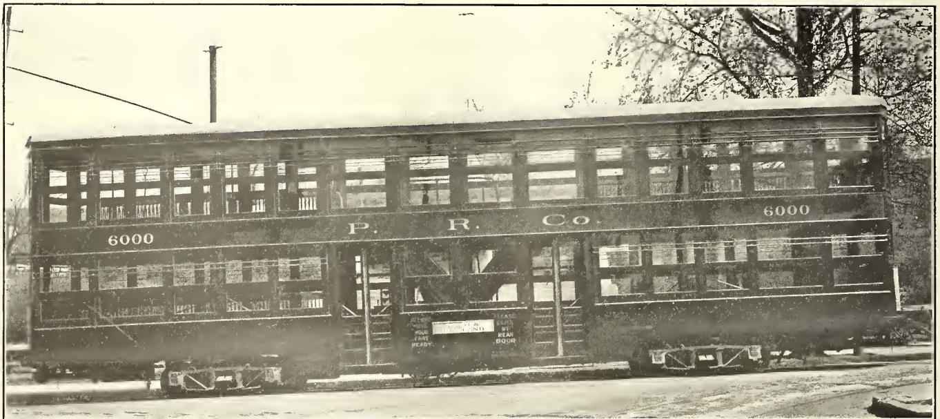
Pittsburgh Double-Deck Cars—View of Original Car Showing Separate Exit and Entrance Doors
