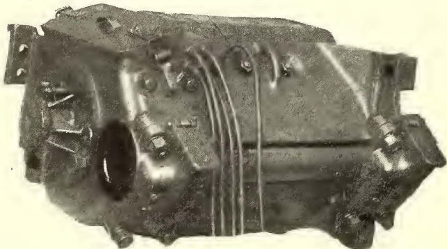
Third Avenue Welding—Commutator End of New Frame No. 57-U Motor
