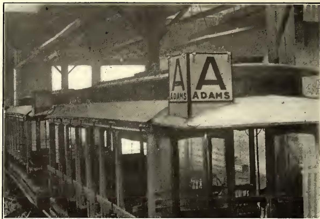
Peoria Route Signs—View of Signs in Place on Cars
