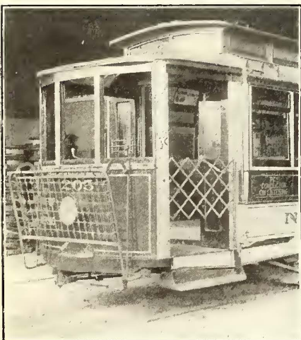
Manually Operated Fender Folded Up at Rear End, in Running Position and Dropped to Rails
