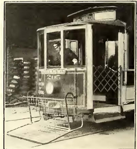
Manually Operated Fender Folded Up at Rear End, in Running Position and Dropped to Rails
