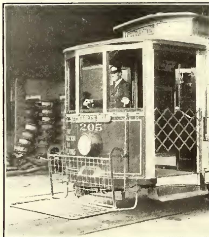
Manually Operated Fender Folded Up at Rear End, in Running Position and Dropped to Rails
