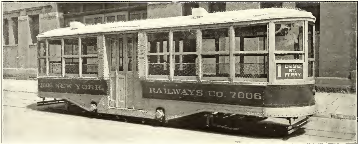
Storage Battery Stepless Car, New York Railways
