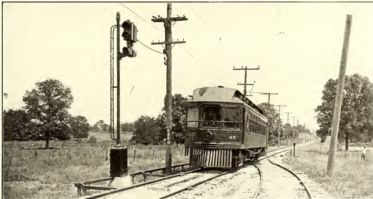
View on Terre Haute, Indianapolis & Eastern, Showing Light Signals for Adjoining Blocks Mounted on One Mast
