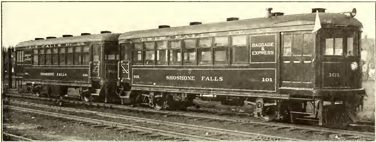
Multiple-Unit Cars with Continental Type Suspension, Used Singly for Passenger Service and Together as a Freight Locomotive
