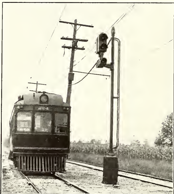
Light Signal with Permissive Indication, Union Traction Company of Indiana
