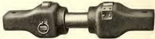
New Automatic Coupler—Coupler Boxes Locked Together
