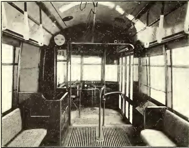
Interior View Showing Conductor's Stand Inside of Car
