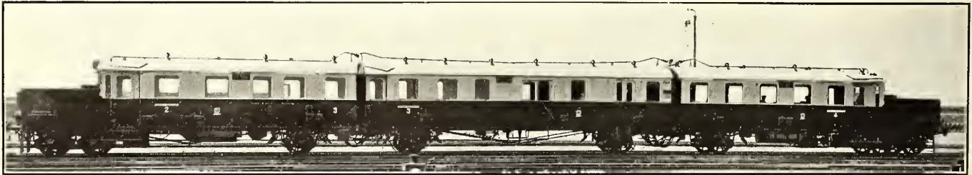
One of the New Triplet Storage Battery Cars, Prussian State Railway
