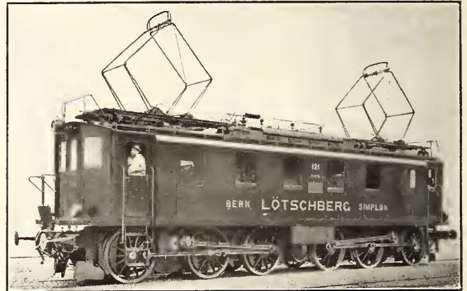
Lötschberg Locomotives—Original 2000-hp Design, in Service Since 1911
