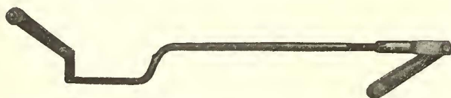
Montreal Cars—Under-Platform Levers with Door Open; Motorman's Handle Shaft at Left and Door-Hinge Shaft at Lower Right-Hand Corner
