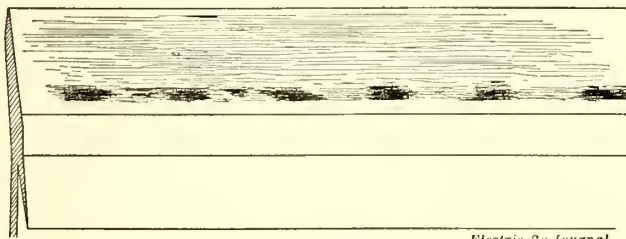
Fig. 3—Rail Corrugation—Beginning of Corrugation
