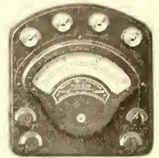
MODEL 280, Triple Range Portable Volt-Ammeter (One-quarter Size.)
