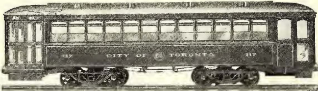
End Platform, Double End, City Car. Length, 45' 1". Weight body, 19,270 lbs. Seating 48.
