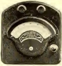
MODEL 280, Single Range Portable Voltmeter. (One-quarter Size.)
