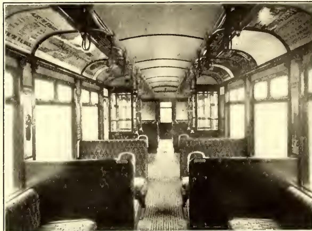
Rapid Transit Progress in London—Interior of Center-Door Car for Metropolitan and District Lines, Showing Glass Wind Shields
