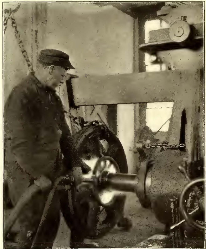
Heat Method for Installing Wheels on Axles, New York, Westchester & Boston Railway
