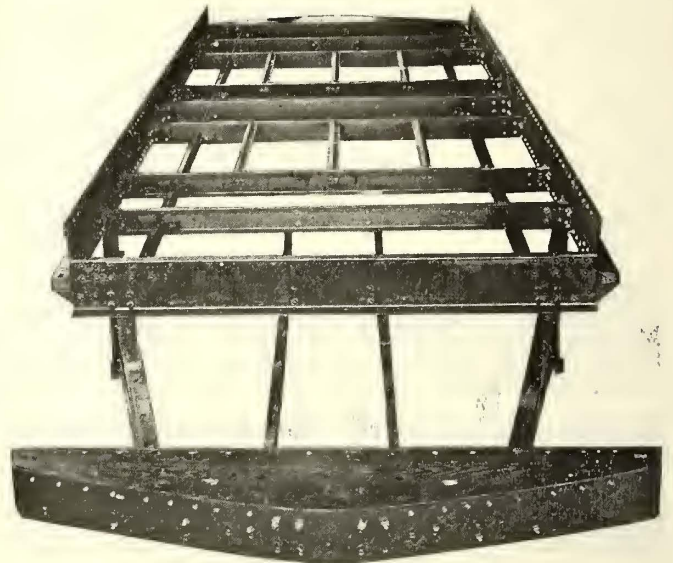
Underframe of Pine Bluff Single-Truck Car
