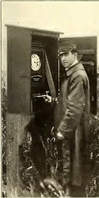
Application of Running-Time Terminal Clocks on an Outlying Line of the British Columbia Electric Railway and on a City Line of the Third Avenue Railway; Also Fac-Simile of Running-Time Card Made with These Clocks on Elevated Lines of Interborough Rapid Transit System
