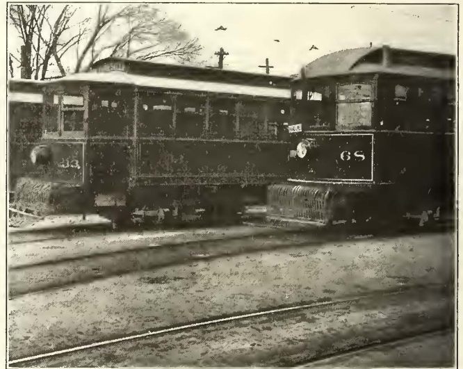
Cleveland, Painesville & Eastern Railroad—Contrast of New and Old Vestibule
