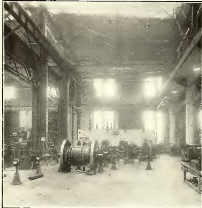
New Haven Shops—View of Armature-Winding Department, with Baking Oven at the Rear
