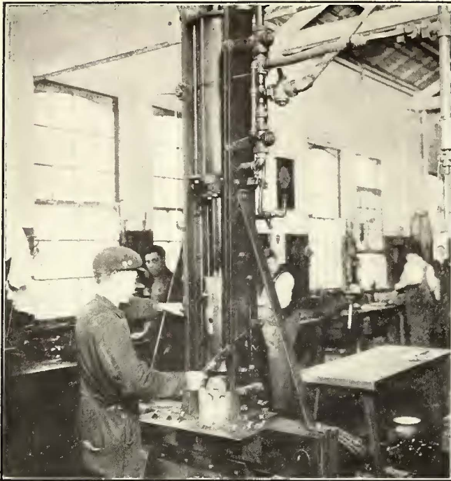
Safety First in New York—Air Hammer with Safety Latch Held Open by Left Hand of Operator
