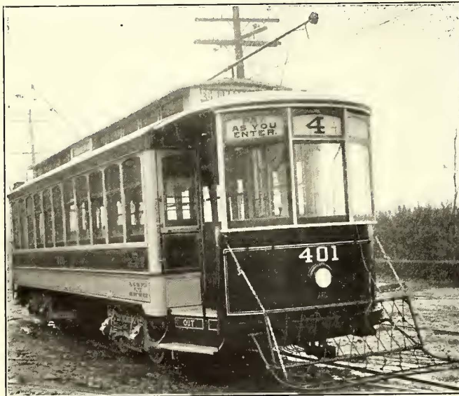
Baltimore Car—View Showing Route Number Sign
