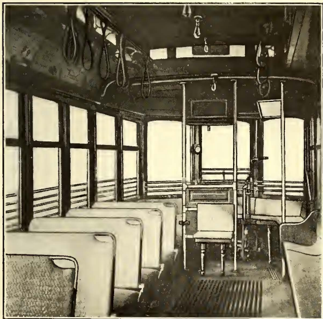
Pittsburgh Car—View Showing Stationary End Seats and Location of Control Handles—Motorman's Mirror Over Right-Hand End Window
