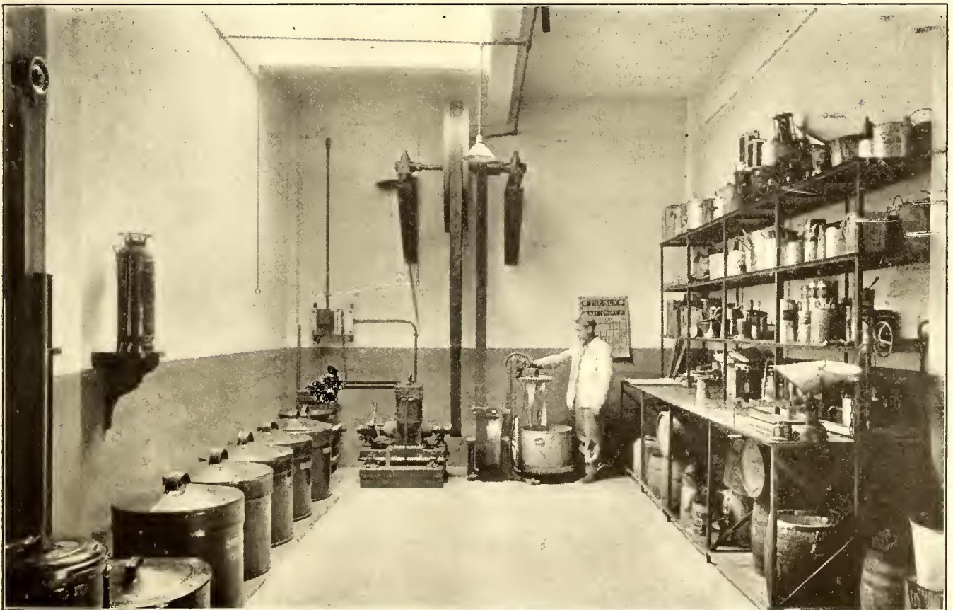
Baltimore Oil House—Mixing Paint by Means of an Old Bi-polar Motor, Belt Drive and Gearing
