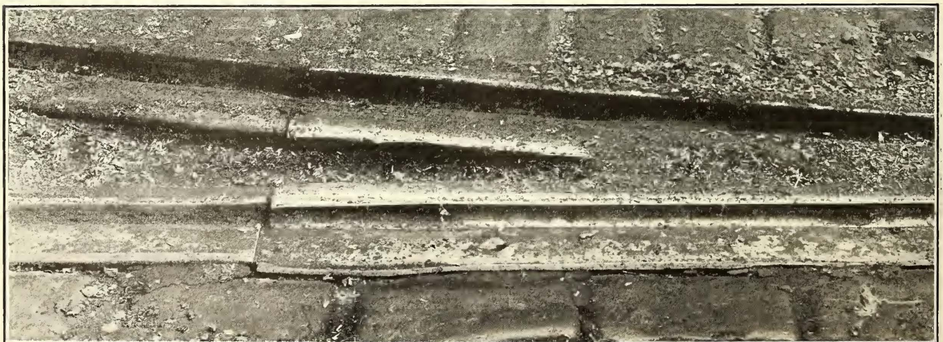
Chicago Special Work—Fig. 1—Showing Cupping of Manganese Mate at Run-off from Chicago Rail, Installed October, 1903; Traffic, 80 Wheels Per Hour
