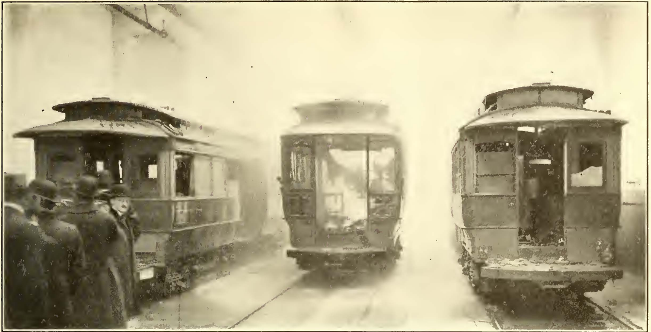
Philadelphia Sprinkler Test—Fig. 4—View Taken After the Sprinkler Had Put Out the Fire Without Giving It a Chance to Spread to the Cars on the Near-by Tracks
