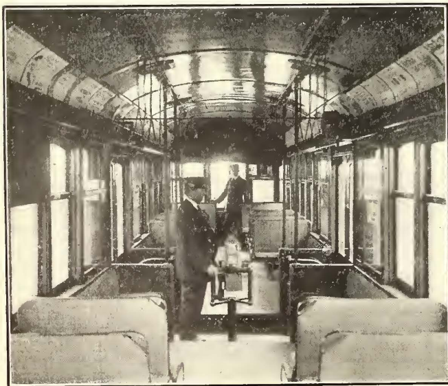
Richmond Center-Entrance Car—Combined Fare-Box Pedestal and Handhold
