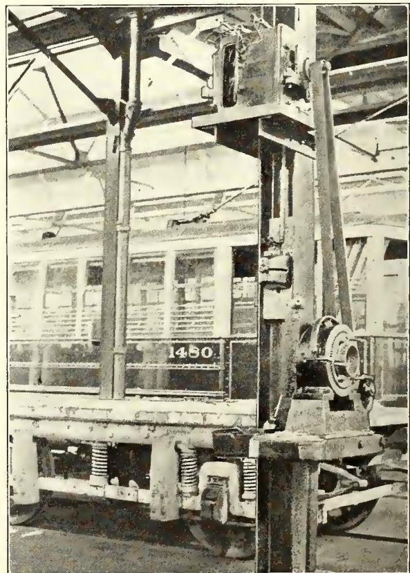
Compact Motor Drive, Montreal Shops
