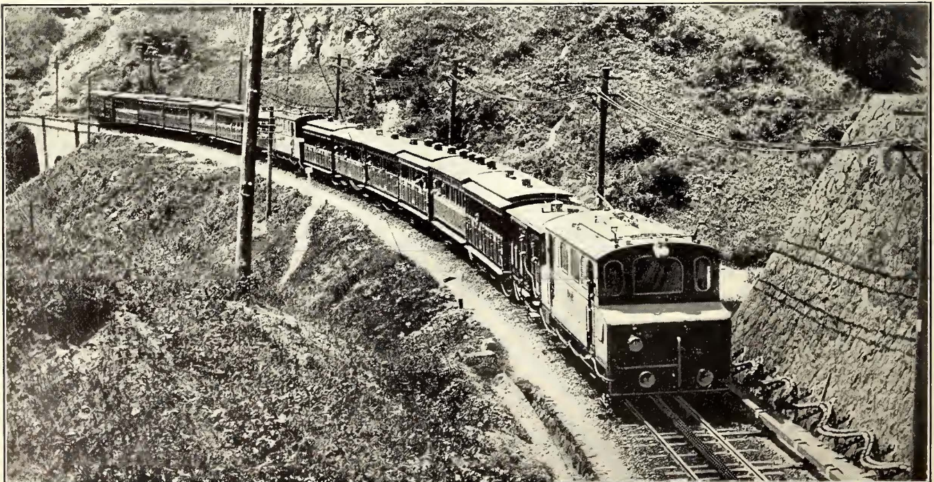
Usui-Toge Railway—Electric Train with Head and Center Locomotives
