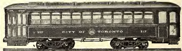
Steel Center Vestibule Double End Interurban Car with Smoking Compt. Length, 48' 0". Weight body, 24,750 lbs. Seating, 60.
