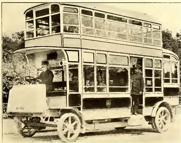
VIENNA SIDE-ENTRANCE BUS OF SPÄNGLER TYPE; NOTE OVERHANG
