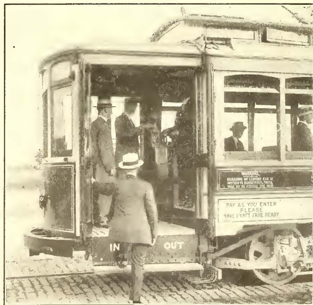
BALTIMORE INCLOSED CARS—REAR ENTRANCE AND EXIT COMBINED, ALSO POSITION OF FARE BOX
