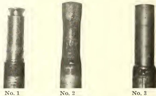
FIG. 1—WORN, WELDED AND FINISHED AXLES OF THIRD AVENUE RAILWAY SYSTEM
