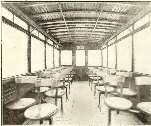
PAIRS OF PIVOTED SEATS ON UPPER DECK OF GLASGOW CAR; NOTE ALSO ABSENCE OF HEADLINING
