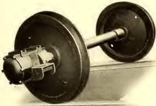
BALL-BEARING JOURNAL BOX FOR STANDARD 0-50 TRUCK— RADIAL LOAD ON EACH JOURNAL 6500 LB.
