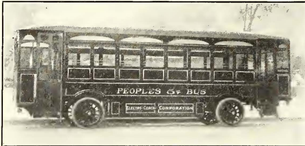
JITNEY BUS—VIEWS OF SEMI-CONVERTIBLE STORAGE-BATTERY BUS PROPOSED FOR NEW YORK
