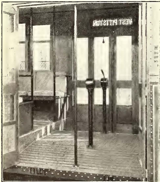
WILKES-BARRE CAR—VIEW AT CENTER, SHOWING RAMP IN WELL, DOOR CONTROL STANDS AND SUPPORTING RAILS; ALSO THE OPEN VESTIBULE WITH CURTAIN ABOVE AND THE FOLDING SEAT ON MOTORMAN'S DOOR
